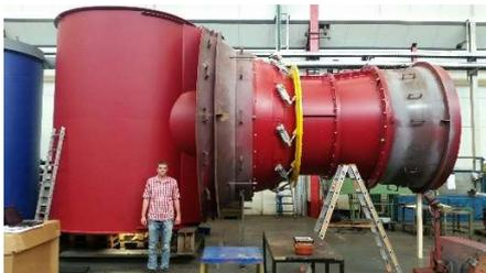
The £5.3m hydropower scheme will use the flow of the River Calder to power a single 500kW axial turbine that will generate around 2.3million units of carbon-free electricity per year, equivalent to the consumption of 800 households. It will run 24/7, 10-11 months of the year, for at least the next 100 years. Salmon, eels and other migratory fish will be able to pass the
